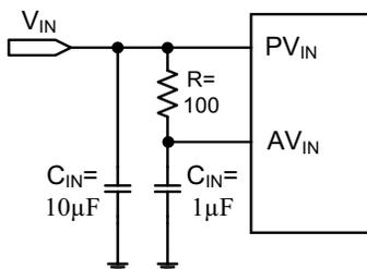
Figure 1: Filtering power supply
